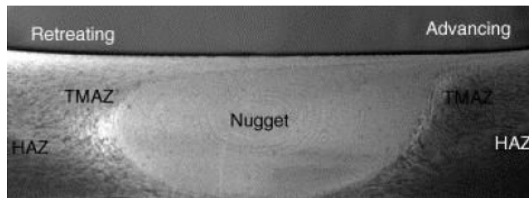
Figure 18. View of the weld with characteristic traces of the “onion slice” effect and deviation in the direction of flow behind the rotating tool (Prabhu et al., 2018)
