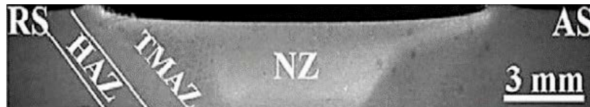
Figure 17. Cross-sectional view of the welded joint AA2009/SiC/17(p) (Ni et al., 2013)
