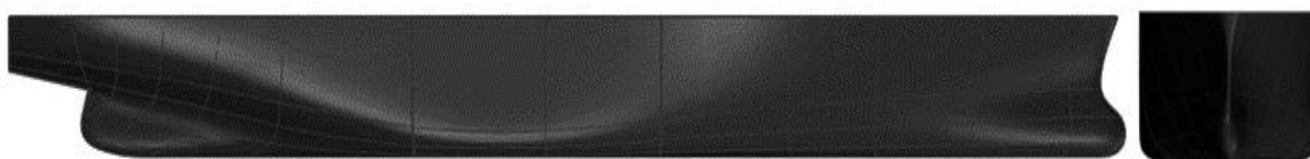
Figure 1. Ship geometry for 192-meter containership
