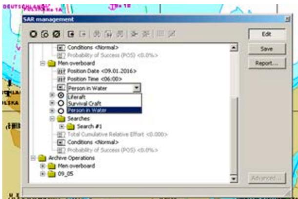
Figure 3. SAR Management window for determining the position of an incident
