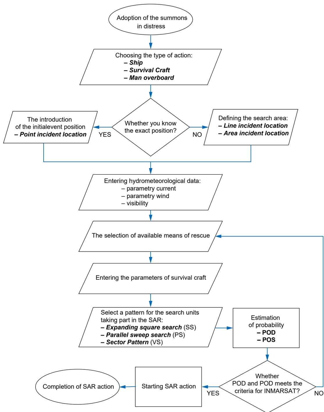
Figure 19. The block diagram of rescue action planning
