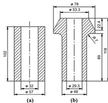
Figure 1. Shape and geometrical dimensions of: (a) a tube-shaped billet, (b) forging with an outer flange
