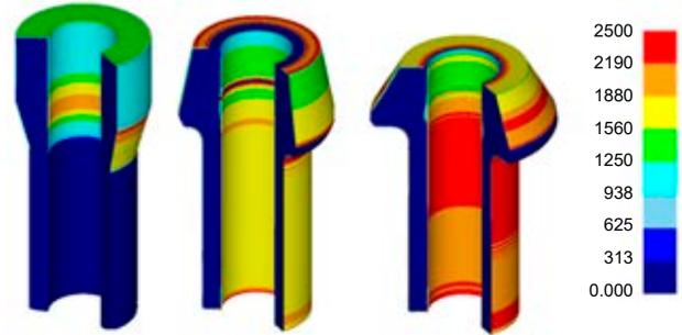
Figure 6. Surface pressure (MPa) distribution in the final phase of each forming stage
