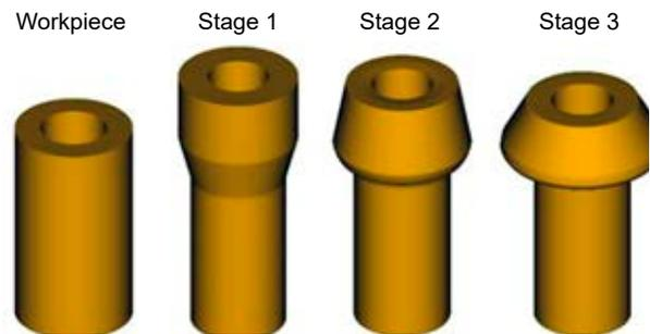
**Figure 3.** Progression of the shape of forgings at each stage of the process
