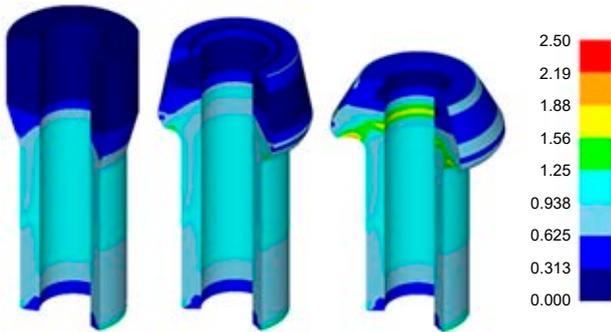
Figure 4. Effective strain distribution in the final phase of each forming stage
