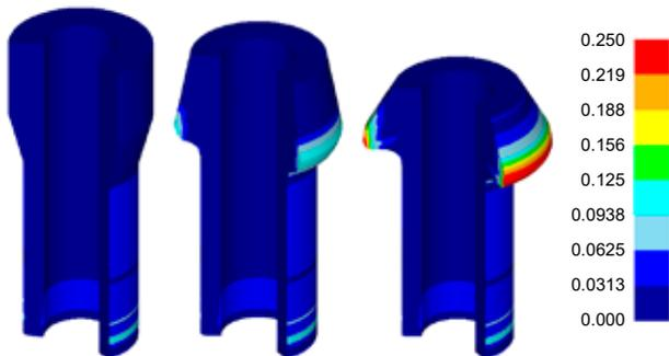
Figure 5. Distribution of the Cockcroft-Latham criterion in the final phase of each forming stage
