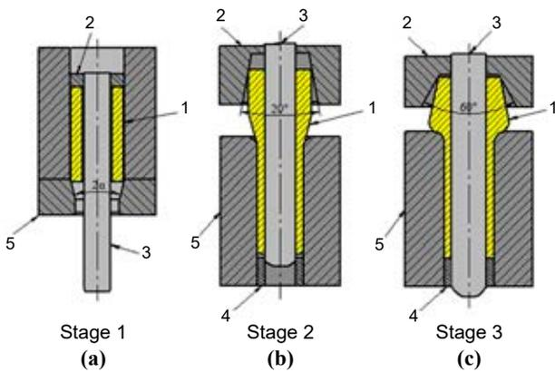
**Figure 2.** Tools for forging hollow elements with a flange: (a) die for extruding the shaft portion and dies for forging the flange with an initial (b) and (c) finished impression; 1 – billet, 2 – punch, 3 – mandrel, 4 – ejector, 5 – die
