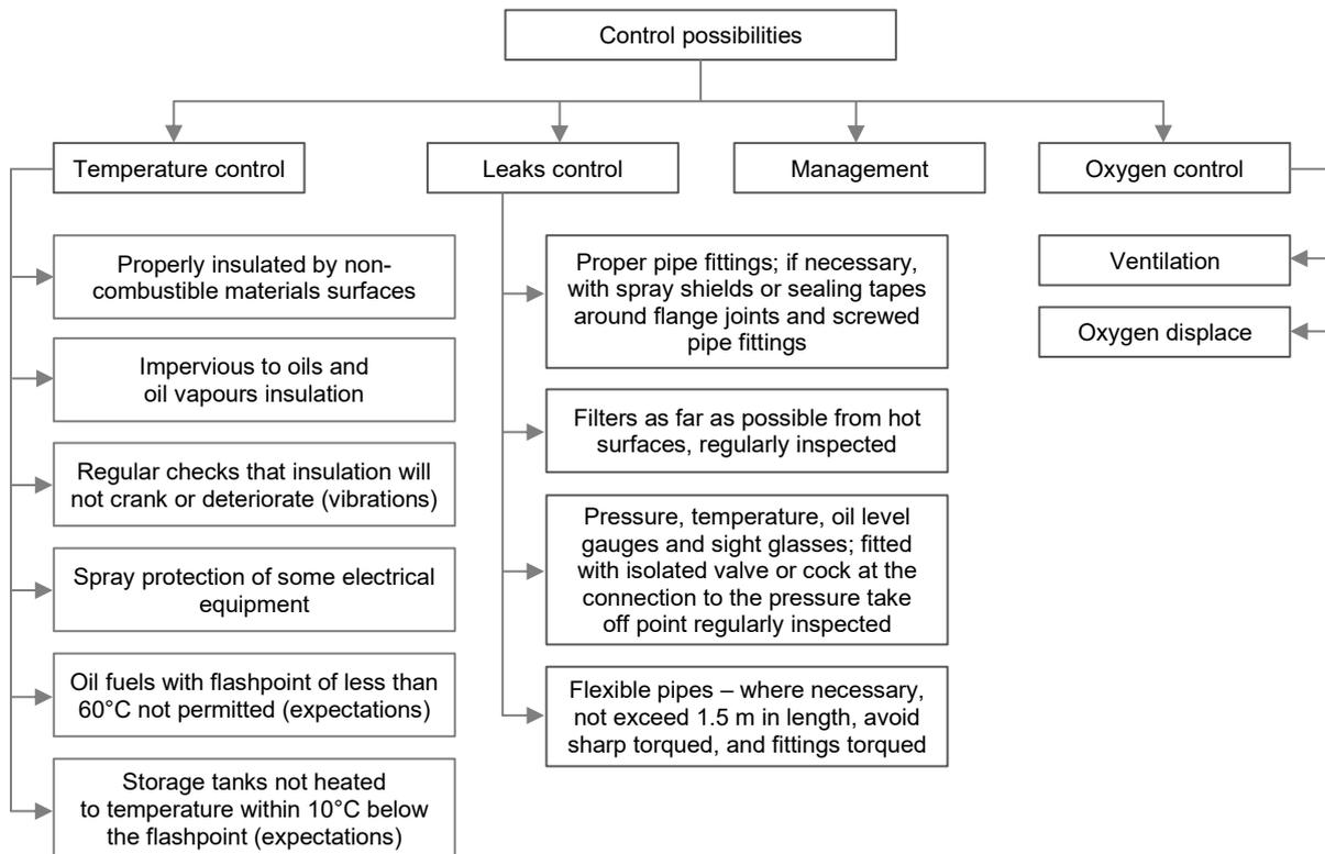
Figure 6. Identification of a fire's origin and spread control possibilities
