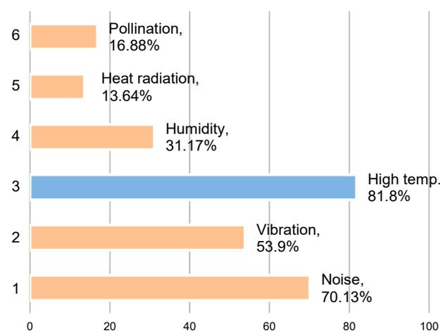
Figure 4. The distribution of factors affecting the work environment in an engine room
