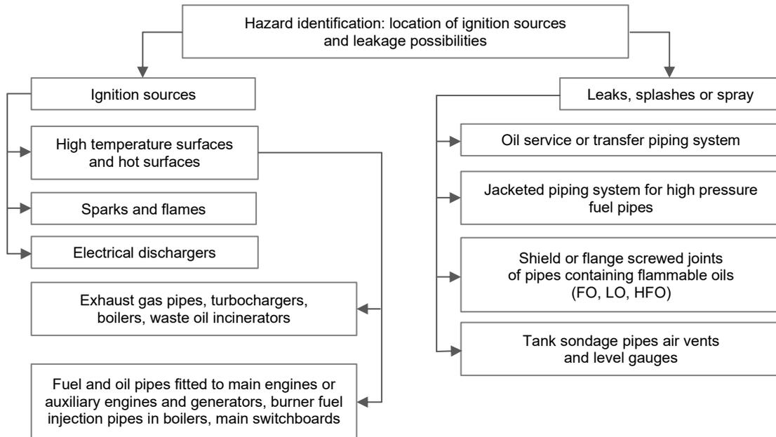
Figure 5. The list of ignition sources and leaks to be checked regularly by the crew
