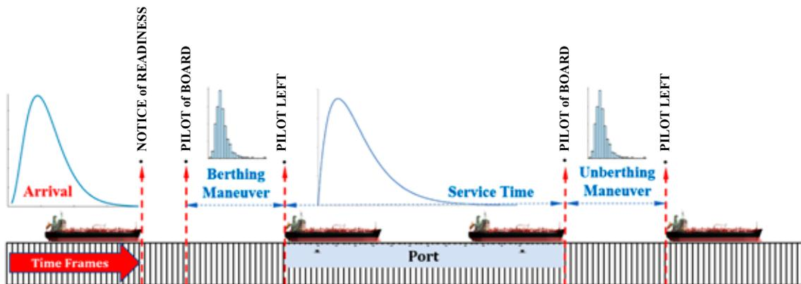
Figure 2. Ship operation processes in a port
