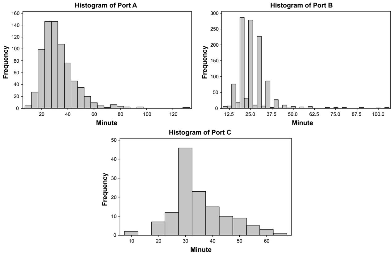
Figure 4. Frequency distributions of the berthing times of class II ships
