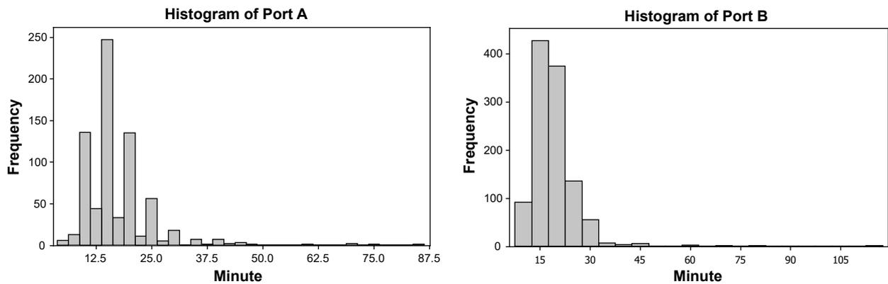
Figure 5. Frequency distributions of the unberthing times of class II ships
