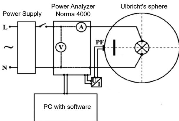
**Figure 2. The diagram of the measuring station for measuring the luminous flux**
