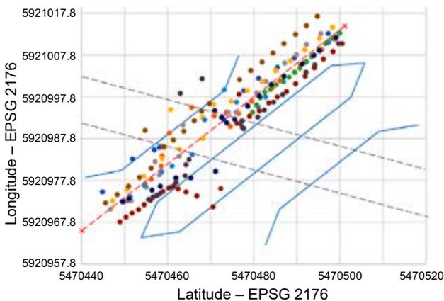
**Figure 5. Positions of vessels passing the Kolejowy Bridge upstream of the river**
