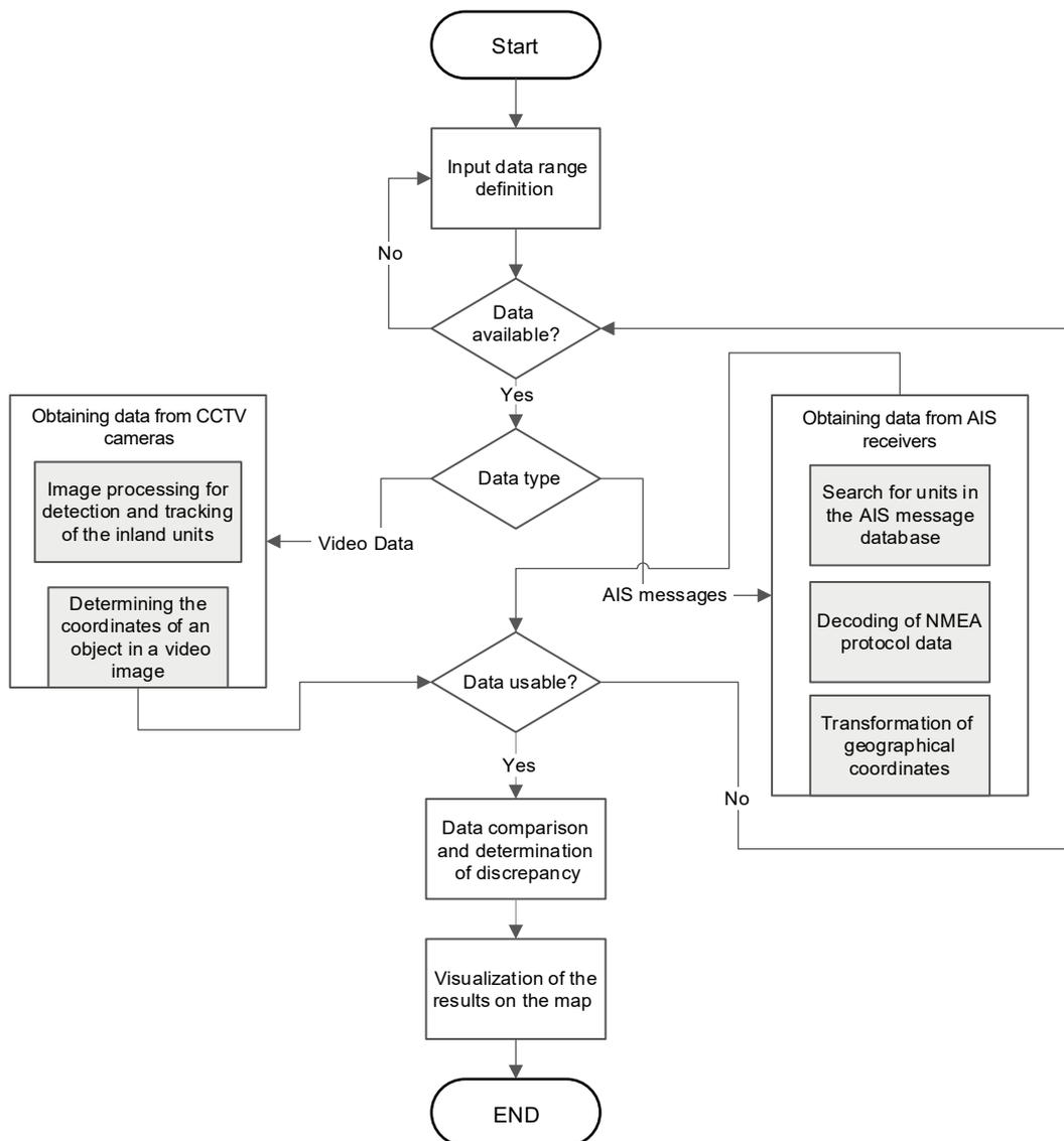
Figure 2. Methodology scheme for inland vessel position analysis
