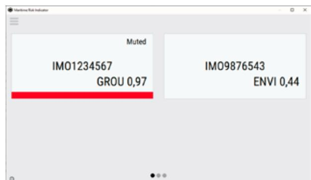
Figure 4. The MRI application running within Windows operating system in a fleet operation center, showing two different vessels “thumbnails” with the most important information in them (vessel ID and the highest risk)
