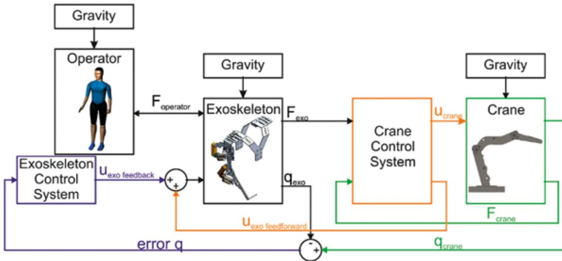
Figure 4. The outline of the mini crane control system
