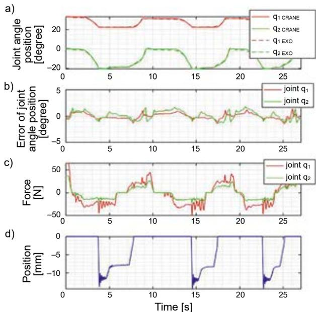
**Figure 10. a) Position of the exoskeleton and mini-crane joints  $q1$  and  $q2$  b) position error c) force measured by the strain gauge beams located on joints  $q1$  and  $q2$  d) depth of penetration into the obstacle by the end tip of the mini-crane during the 2<sup>nd</sup> scenario of the experiment using the mini-crane control system with force feedback and feedforward structure**
