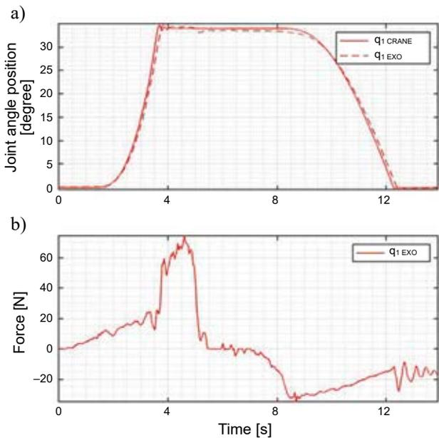
**Figure 8. a) Exoskeleton joint and mini-crane joint position and b) the force measured by the strain gauge beam during the 1<sup>st</sup> scenario of the experiment using the mini-crane control system with force feedback and feedforward structures**
