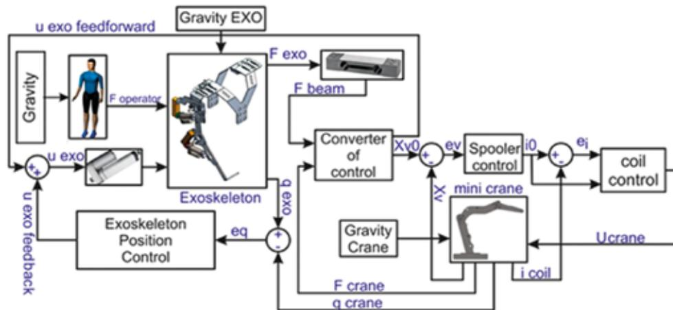
Figure 5. Diagram of the extended intuitive control system of a mini-crane
