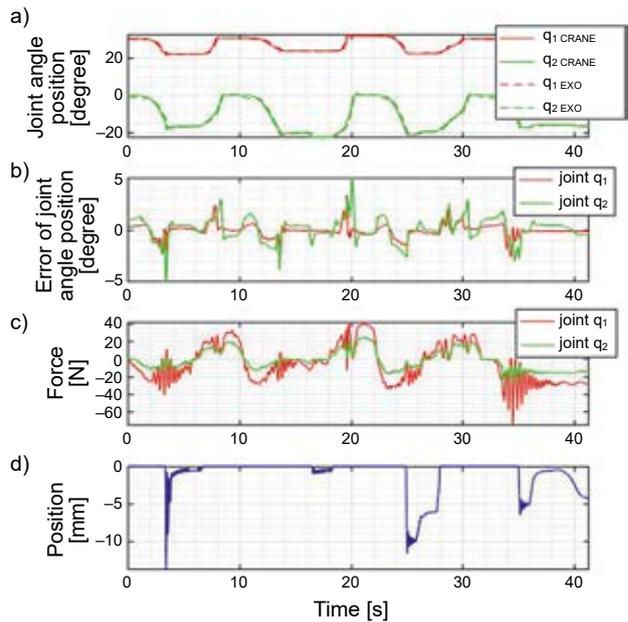
**Figure 9. a) Position of the exoskeleton and the mini-crane joints  $q1$  and  $q2$  b) position error c) force measured by the strain gauge beams located on joints  $q1$  and  $q2$  d) depth of penetration into the obstacle by the end tip of the mini-crane during the 2<sup>nd</sup> scenario of the experiment using the mini-crane control system with force feedback structure**
