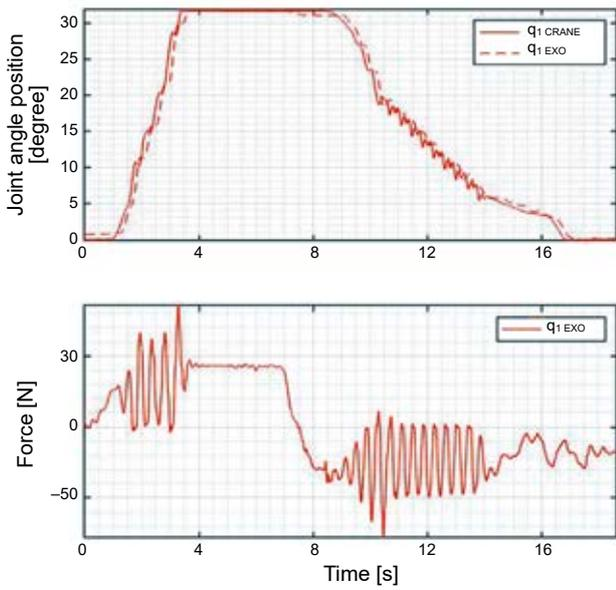
**Figure 7. a) Exoskeleton joint and mini-crane joint position and b) the force measured by the strain gauge beam during the 1<sup>st</sup> scenario of the experiment using the mini-crane control system with force feedback structure**
