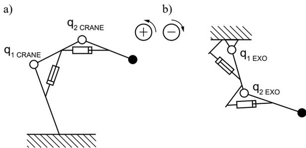
Figure 2. Diagram of the kinematic structure of a) the Slave system and b) the Master system
