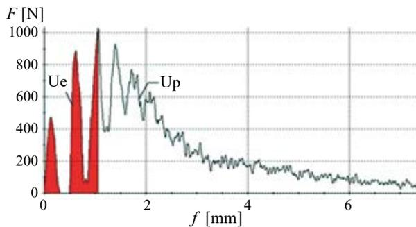
Figure 4. Force-strain diagram  $F(f)$  for a sample with 10% recyclate content and  $\leq 1.2$  mm granulation, obtained during dynamic three-point bending with a Charpy pendulum type shuttle hammer, where: Ue – operation in the elastic state, Up – work related to the development of defects
