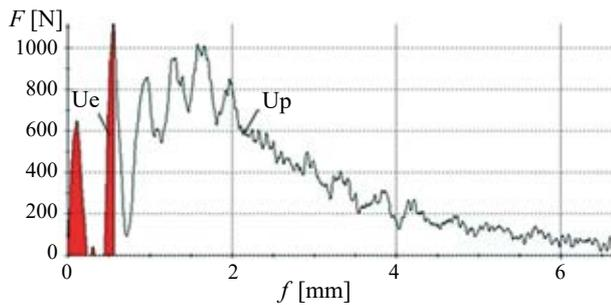
Figure 3. Force-strain diagram  $F(f)$  for samples with 0% recyclate content obtained during dynamic three-point bending on a Charpy type pendulum hammer, where: Ue - operation in the elastic state, Up - work related to the development of defects
