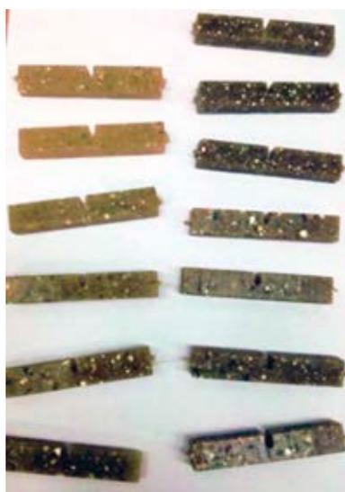
**Figure 1. Charpy impact test specimens with 'U' type notch with 10% and 20% recycle content**
