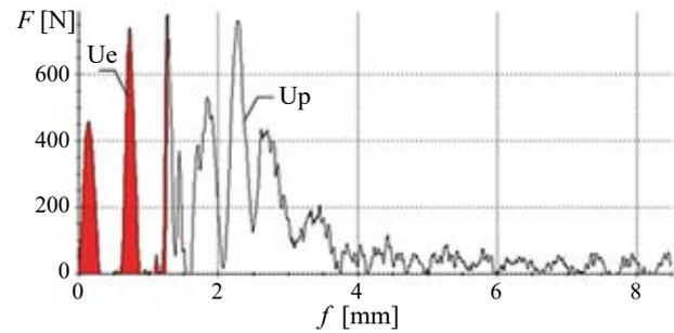
Figure 5. Force-deformation plot  $F(f)$  for a sample with 20% recyclate content, granulation of  $\leq 1.2$  mm, obtained during dynamic three-point bending with a Charpy pendulum type shuttle hammer, where: Ue - operation in the elastic state, Up - work related to the development of defects
