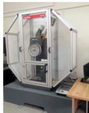
**Figure 2. Swinging hammer, model RKP450 from Zwick Roell**
