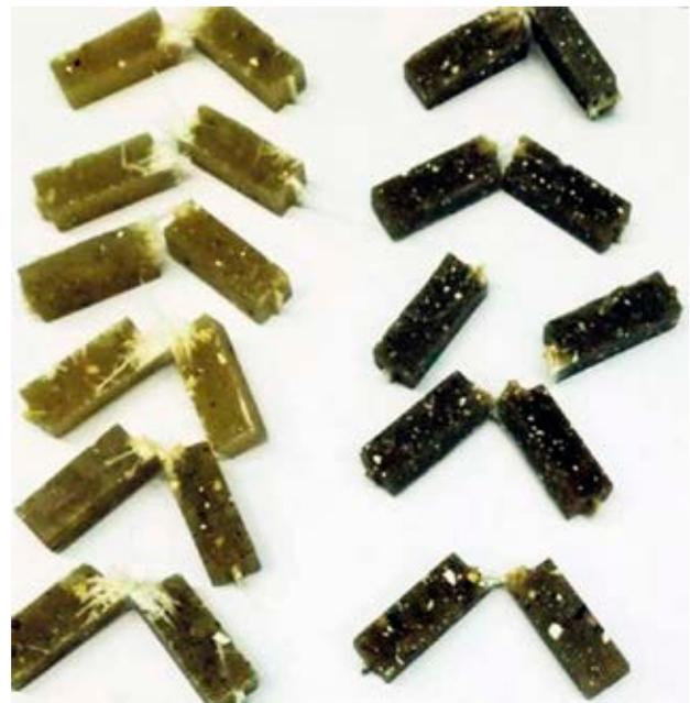
Figure 6. Scrap samples with 10% and 20% recyclate content, obtained as a result of dynamic bending
