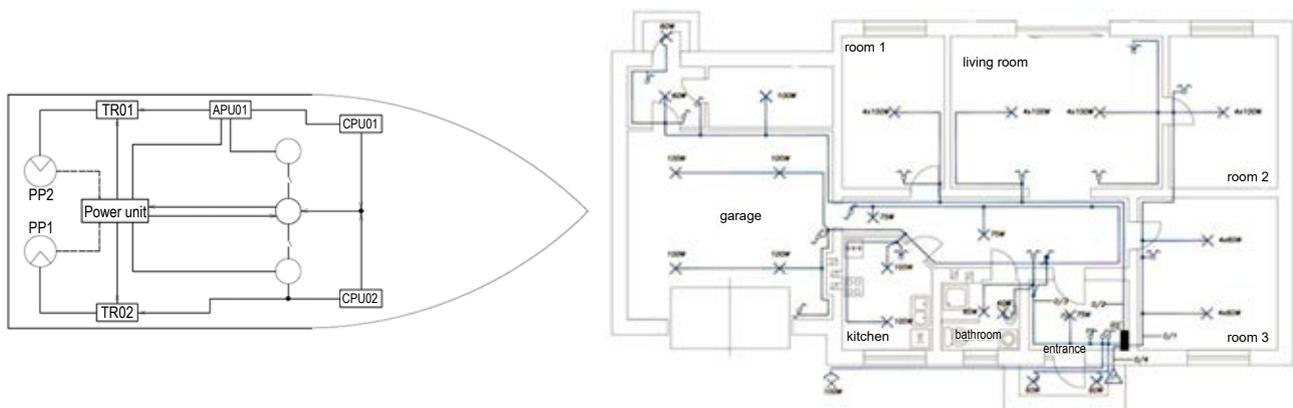
**Figure 3. Wiring diagram of an exemplary boat and a residential house**
