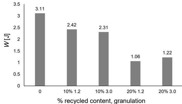
Figure 5. The effect of recyclate content % and granulation on energy (W)
