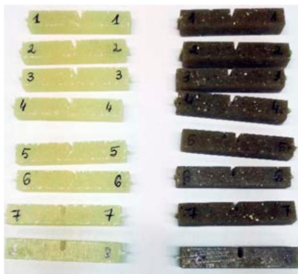
Figure 1. Charpy impact test specimens
