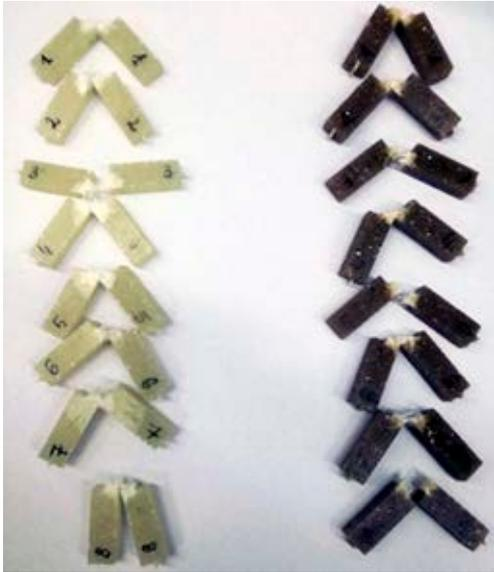
Figure 3. Samples after Charpy impact test
