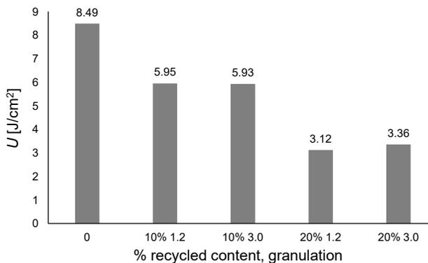
Figure 4. Impact of recyclate content % and granulation on impact resistance [J/cm<sup>2</sup>]
