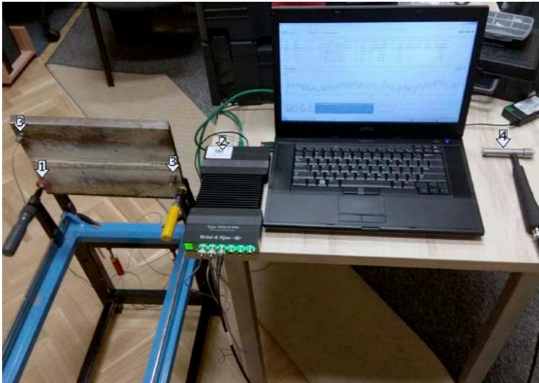
**Figure 1.** Stand for testing welded joints using vibration methods. The stand includes: 1– rack, in which plates (welding samples) could be mounted horizontally – four-point mounting or vertical – two-point mounting, 2 – Bruel & Kjaer type 3050-A-vibration analyzer 60, 3 – accelerometers 4514-B, 4 – modal hammer (8206-002) with three exchangeable tips, i.e. metal, silicon and Teflon
