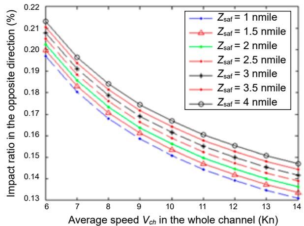
**Figure 9. The impact ratio in the opposite direction for an LNG ship’s safety zone**
