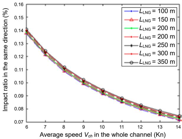
**Figure 6. The impact ratio in the same direction for different lengths of an LNG ship**
