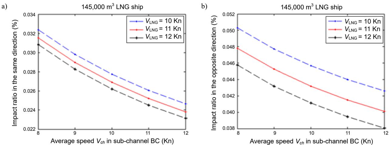
Figure 3. The impact ratio on sub-channel BC, a) Impact ratio in the same direction, b) Impact ratio in the opposite direction
