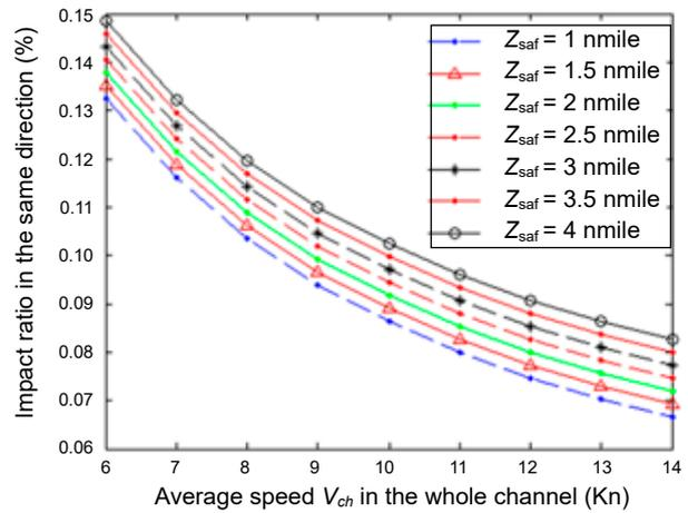
**Figure 8. The impact ratio in the same direction for an LNG ship’s safety zone**
