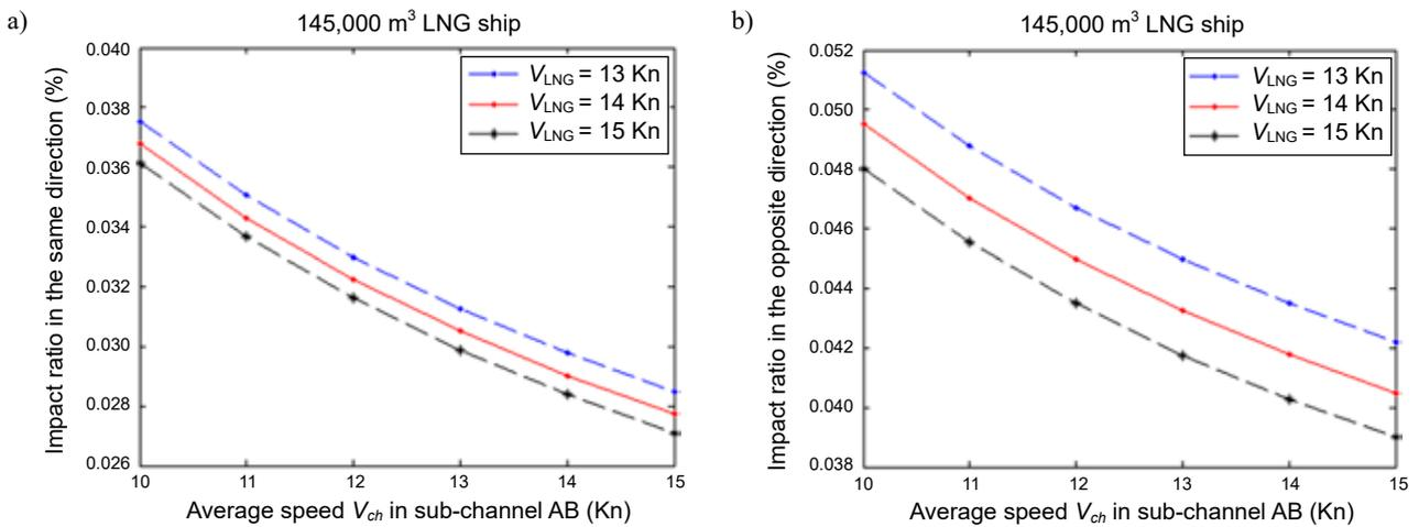
Figure 2. The impact ratio on sub-channel AB, a) Impact ratio in the same direction, b) Impact ratio in the opposite direction
