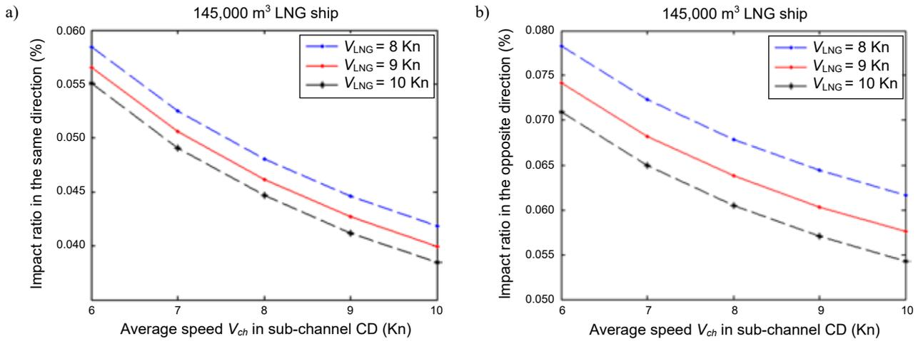
Figure 4. The impact ratio on sub-channel CD, a) Impact ratio in the same direction, b) Impact ratio in the opposite direction
