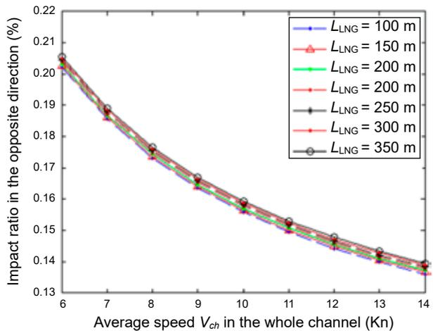
**Figure 7. The impact ratio in the opposite direction for different lengths of an LNG ship**
