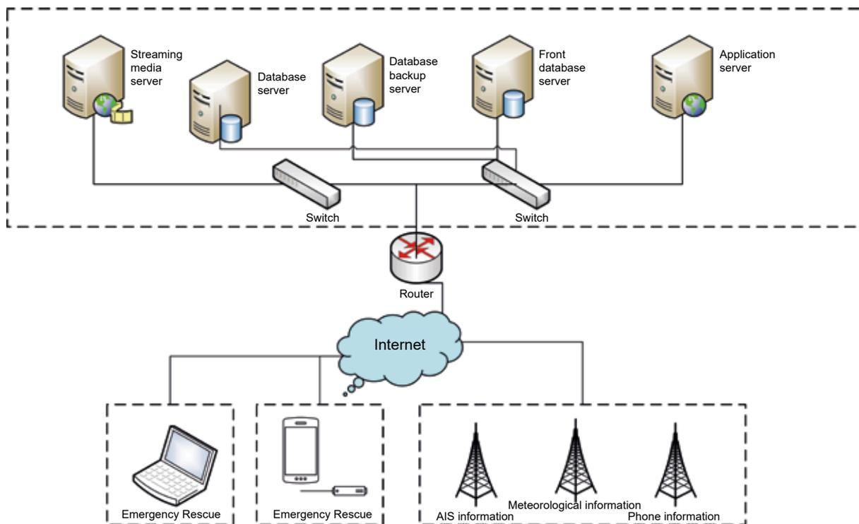
Figure 3. Hardware system composition
