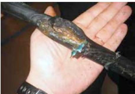
Figure 3. An example of cable damage caused by fishing gear (Carter et al., 2009)
