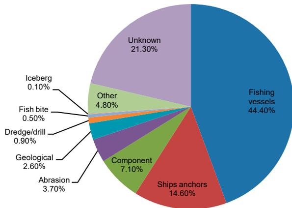
**Figure 1. Underwater cables damage statistics. Data collected by the Department of the Interior, Bureau of Ocean Energy Management, 2014**
