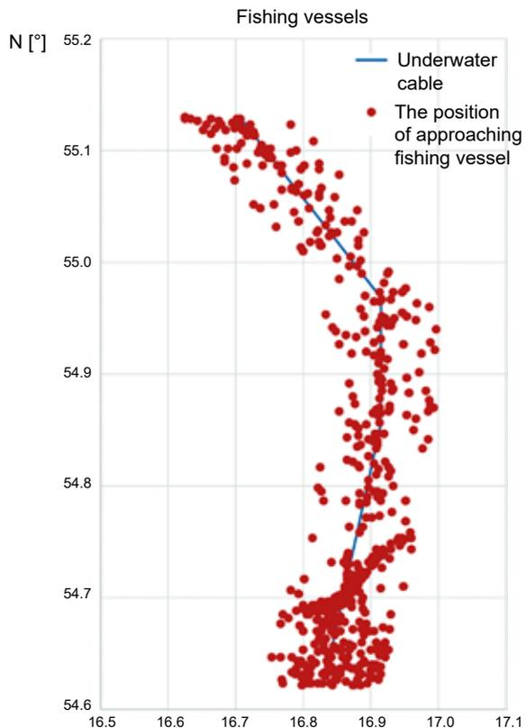
Figure 7. Closing fishing boats situations to underwater cable independently boat speed. VMS data
