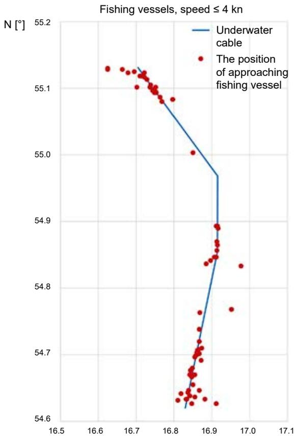
**Figure 8. Closest position of fishing vessels to the underwater cable (distance less than 3 Nm, speed less than 4 knots)**
