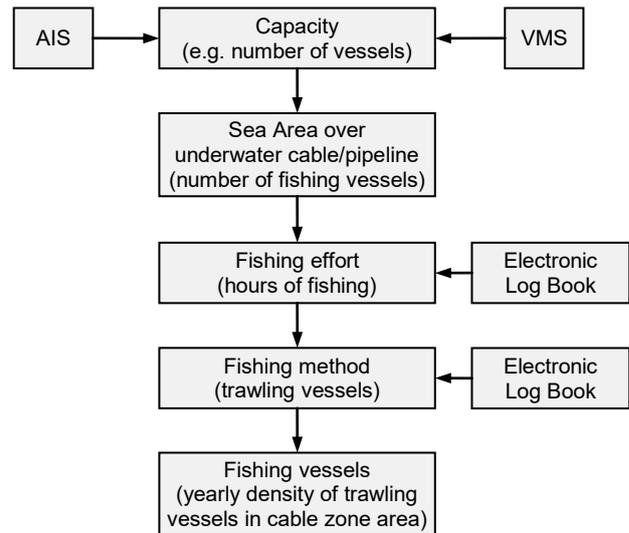
Figure 5. Scheme for estimating which trawling fishing vessels are a danger to underwater cables
