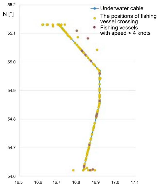
**Figure 9. Positions of fishing vessels passing over the underwater cable from the AIS data**
