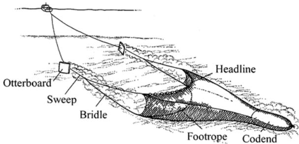
Figure 2. Schematic diagram of an otter trawl (Palanques, Guillen & Puig, 2001)
