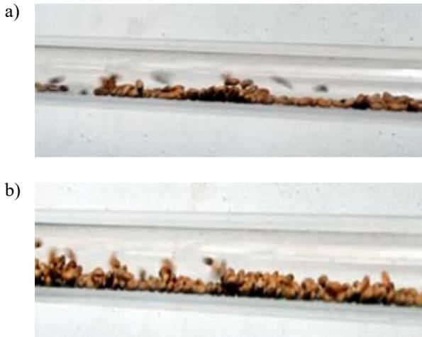
Figure 6. Image of flow structure during the horizontal pneumatic transport of wheat grains: a) layer moving by sliding b) saltation beginning
