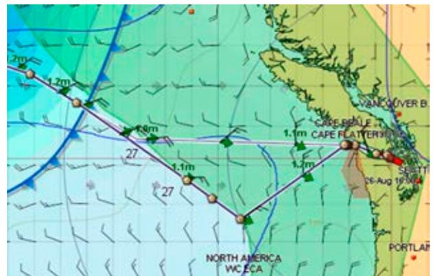
Figure 10. Route leading through the ECA Zone, optimized in the BV system (bold) and route programmed manually (Applied Weather Technologies, 2014)
