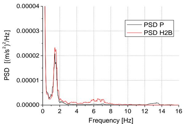
Fig. 8. Comparison between the PSD values of the vertical accelerations of the vehicle floor (P) and the dummy's torso (H2B)
