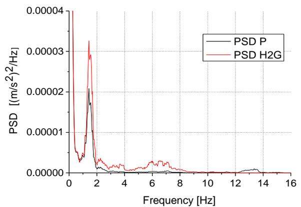
Fig. 7. Comparison between the PSD values of the vertical accelerations of the vehicle floor (P) and the dummy's head (H2G)
