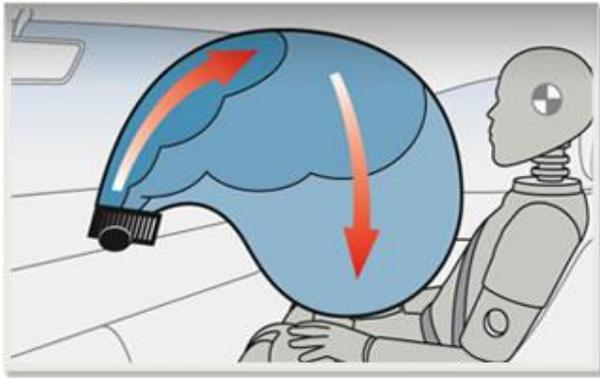
Fig. 3. Example of a special shape of the airbag [16]
