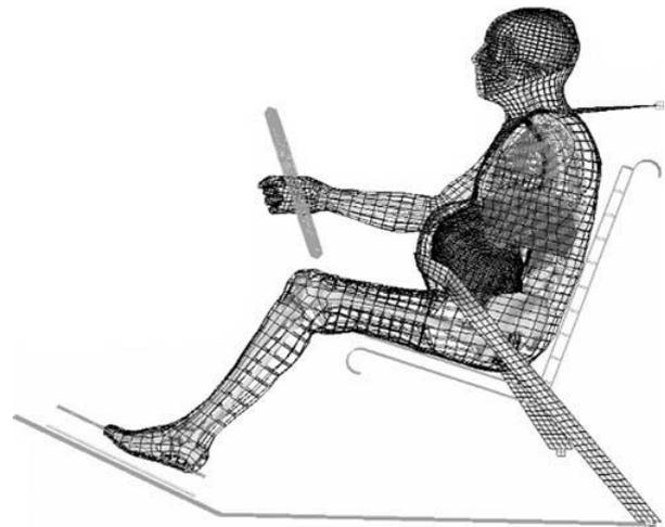
Fig. 5. Side view of a pregnant driver represented by a computer model [30]
