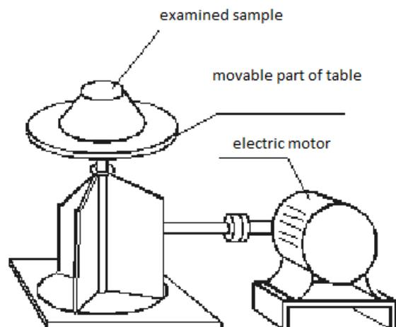
Fig. 1. “Flow Table” method for determining FMP in concentrates (own study based on [2])
