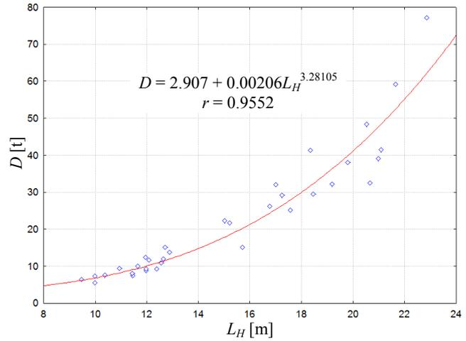
Fig. 7. Full displacement  $D$  depending on length of the hull  $L_H$
