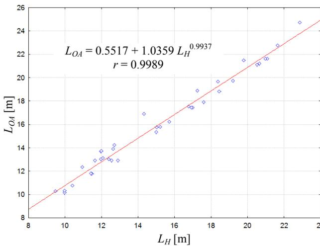
Fig. 2. Length overall  $L_{OA}$  depending on length of the hull  $L_H$
