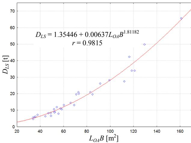
Fig. 6. Displacement of the light ship  $D_{LS}$  depending on the surface of the deck  $L_{OA}B$
