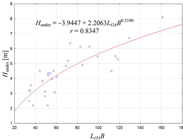
Fig. 4. Height of topside  $H_{\text{under}}$  depending on the surface of the deck  $L_{OA}B$
