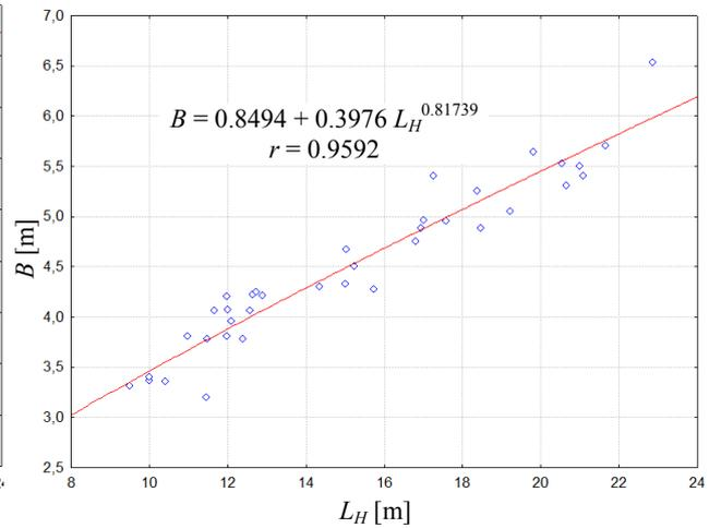
Fig. 3. Breadth  $B$  depending on length of the hull  $L_H$
