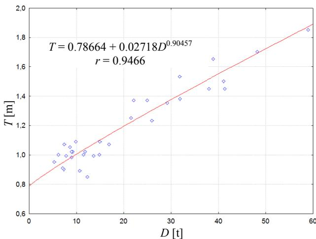
Fig. 8. Draft  $T$  depending on the full displacement  $D_{calc}$
