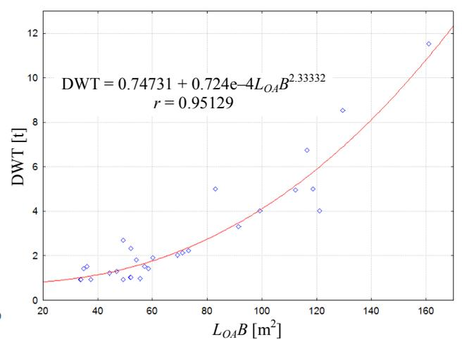
Fig. 9. Deadweight DWT depending on the surface of the deck  $L_{OA}B$
