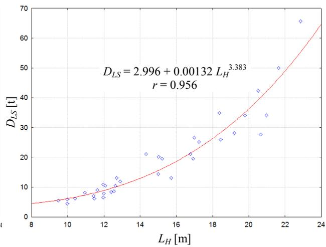
Fig. 5. Displacement of the light ship  $D_{LS}$  depending on length of the hull  $L_H$
