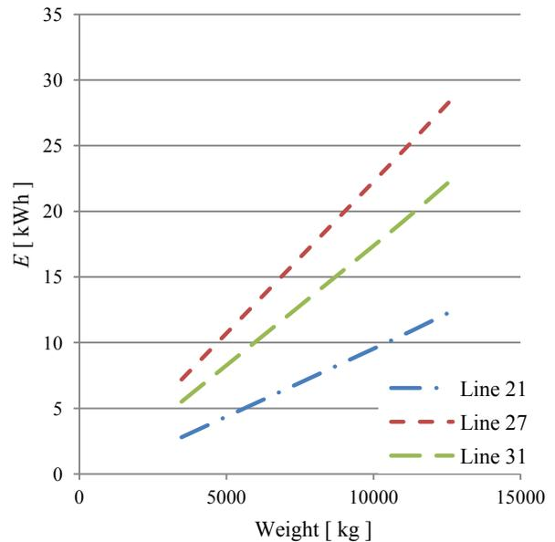
Fig. 11. Course of the energy required to pass the cycle  $E$  – 50% occupation
