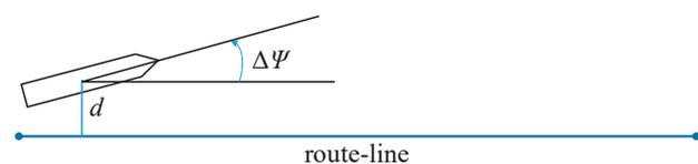
**Figure 1.** General task of the adaptive neuroevolutionary autopilot is to keep the vessel as close as possible to defined route-line ( $d \rightarrow \min$ ) with the smallest course changes ( $\Delta\Psi \rightarrow \min$ )
