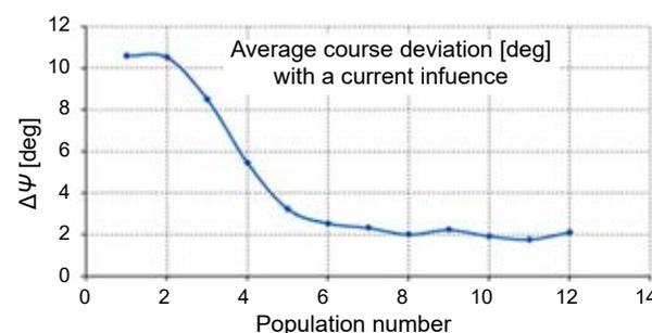
**Figure 5. Average course-over-ground deviation of the ferry, divided in 12 groups of 50 measurements of best helmsmen, with environmental disturbances from a water current**
