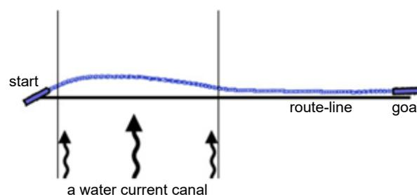
**Figure 6. Trace route of the vessel with a water current canal influencing her maneuvers**
