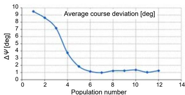
**Figure 4. Average course-over-ground deviation of the ferry, divided in 12 groups of 50 measurements of best helmsmen, without environmental disturbances**
