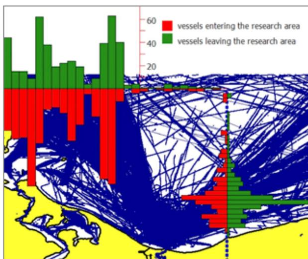
Figure 3. Ships crossing the reporting lines in the VTS Świnoujście area a) crossing northern reporting line, b) crossing eastern reporting line (ingoing ships in the area – green, outgoing ships – pink)
