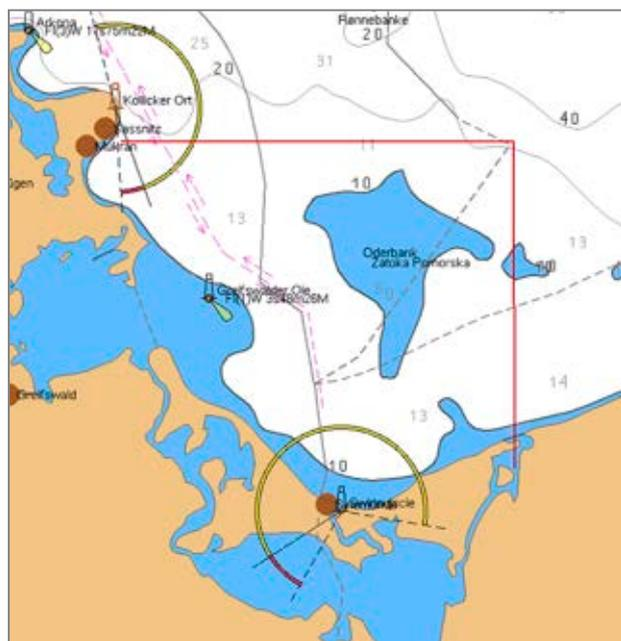
Figure 1. The reporting lines and VTS Świnoujście coverage area (Transas ECDIS NS 4000)
