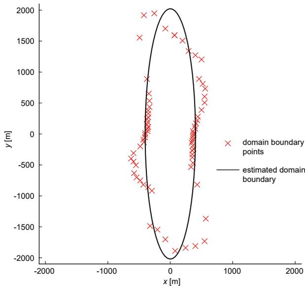
Figure 5. Passenger ship domain in Świnoujście approach area (2A)
