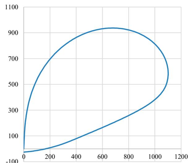
Figure 7. Ship's trajectory during the Anderson turn manoeuvre
