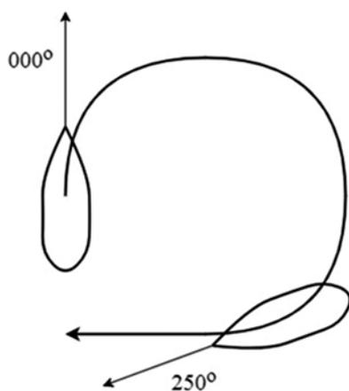
Figure 3. Example of single turn manoeuvre execution
