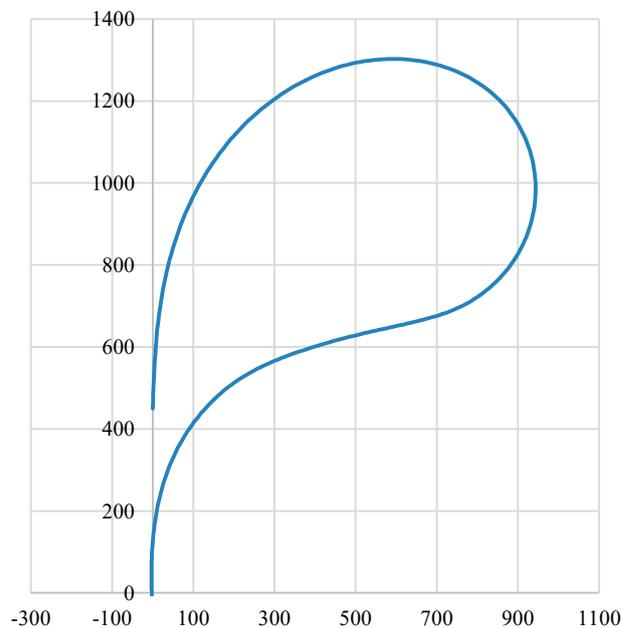
Figure 6. Ship's trajectory during the Scharnov turn manoeuvre
