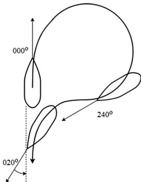
Figure 2. Example of Scharnov turn manoeuvre execution
