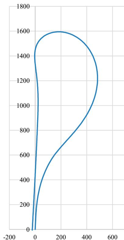
Figure 5. Ship's trajectory during the Williamson turn manoeuvre
