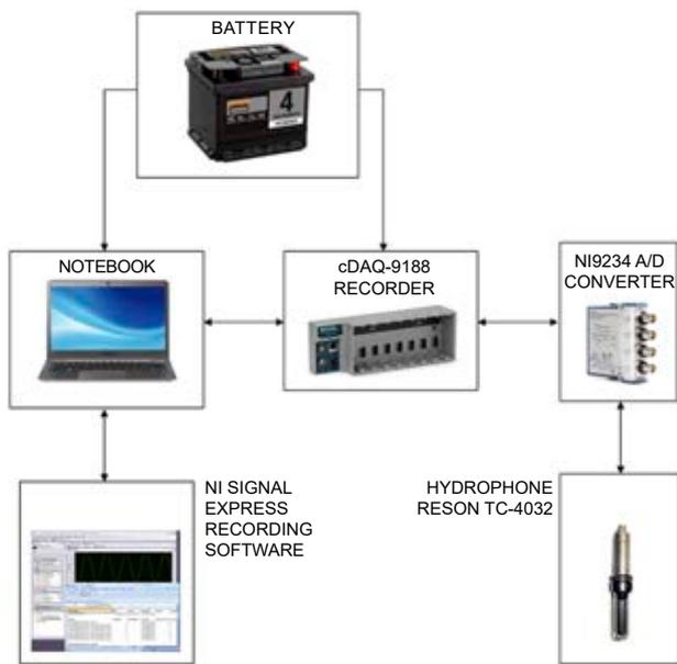
Figure 1. Underwater noise measurement system scheme
