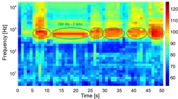
**Figure 8.** OTO spectrogram of underwater vehicle with electric propellers
