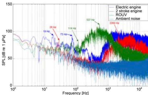
**Figure 5. Narrow band spectrum for the three types of vehicles**
