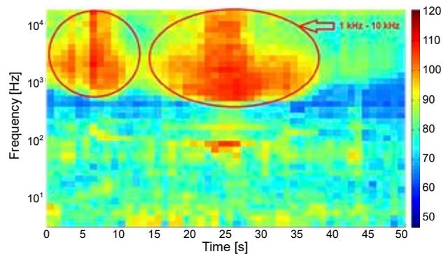
**Figure 6. OTO spectrogram of water surface vehicle with two-stroke engine**
