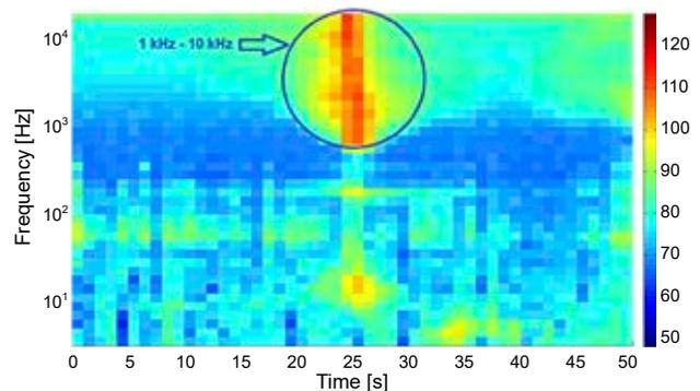
**Figure 7. OTO spectrogram of water surface vehicle with electric engine**
