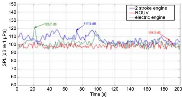
**Figure 4. Sound pressure level generated by three types of vehicles with respect to time**
