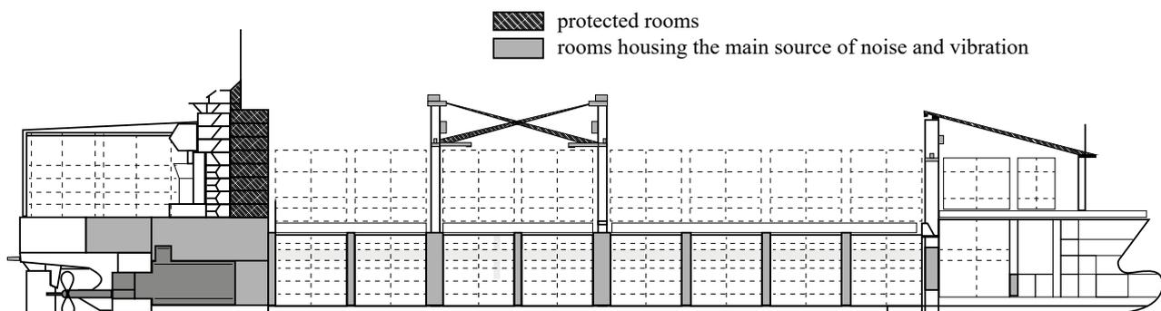
**Figure 8.** Layout of ship rooms (Marczak, 2009)
