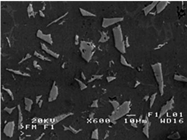
Figure 2. Structure of the composite AlSi9 – 20% SiC (Grabian, 2012)
