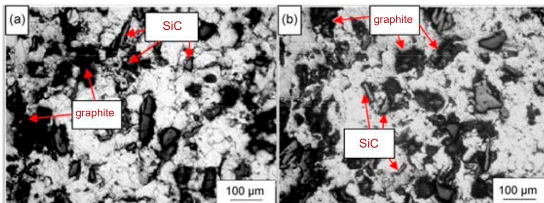
Figure 4. Hybrid composite (a) Al2024/5%SiC/5% graphite, (b) Al2024/5%SiC/10% graphite (Ravindran et al., 2012)
