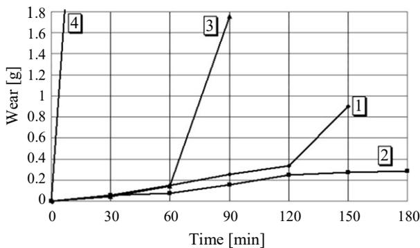
Figure 3. The abrasive wear of materials under dry friction conditions, description of curves in the paper (Grabian, Gawdzińska & Glowacki, 2004)
