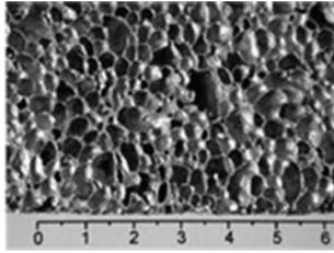
**Figure 6.** Foamed composite material AlSi9-SiC, made at the Maritime University of Szczecin (measurement unit = 1 cm) (own elaboration)
