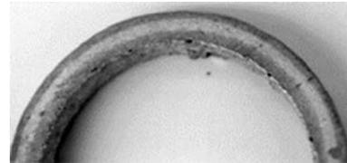
Figure 5. Hybrid bearing with two layers enriched with SiC (outer layer) and graphite (inner layer) AlSi7Mg/15% SiC by volume/5% graphite by volume (Sobczak & Wojciechowski, 2002)
