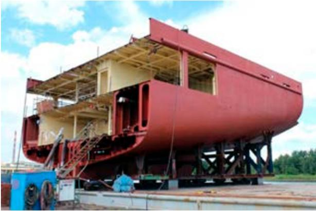
Figure 9. Layout of walls and decks on the cross-section of the hull (Grabian, 2012)
