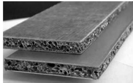
**Figure 7.** Panel: polyester–glass composite/aluminium–ceramic composite foam/glass polyester–glass composite, made at the Maritime University of Szczecin (own elaboration)
