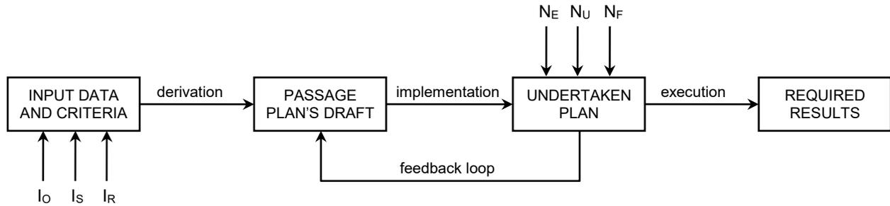
Figure 2. Block algorithm of passage planning
