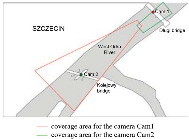
Figure 2. Visibility of CCTV cameras on the Długi Bridge and Kolejowy Bridge in Szczecin
