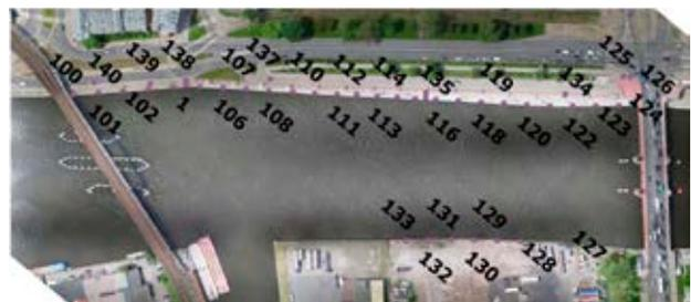
Figure 4. Digital orthophotomap developed on the basis of UAV flights with photopoints measured using a GNSS receiver with RTK correction
