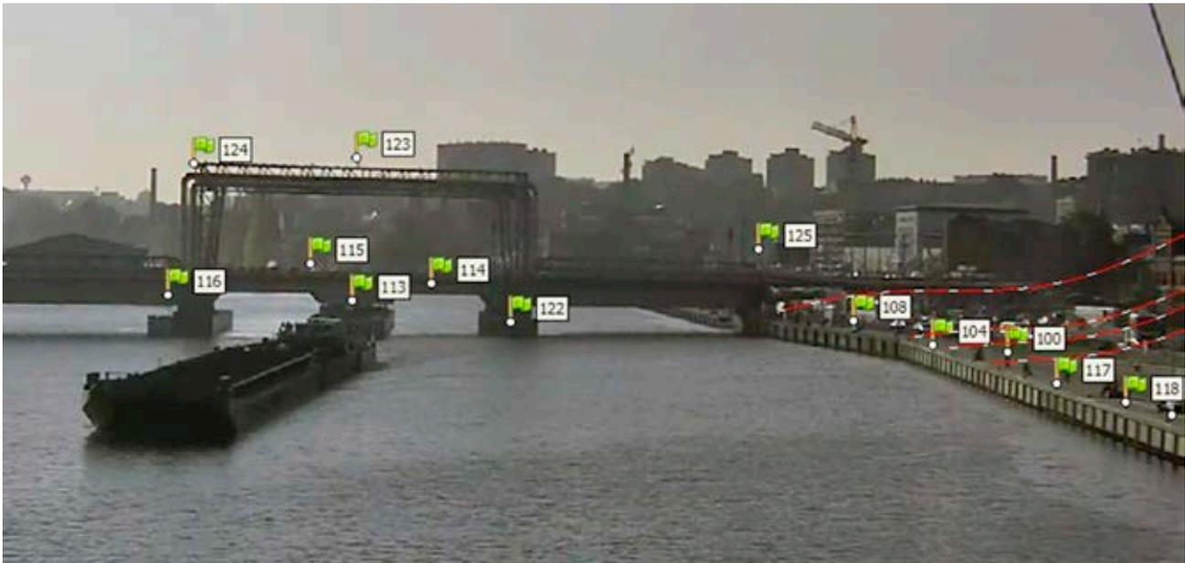
Figure 5. Calibration of the non-metric camera based on the points measured by an electronic tachymeter
