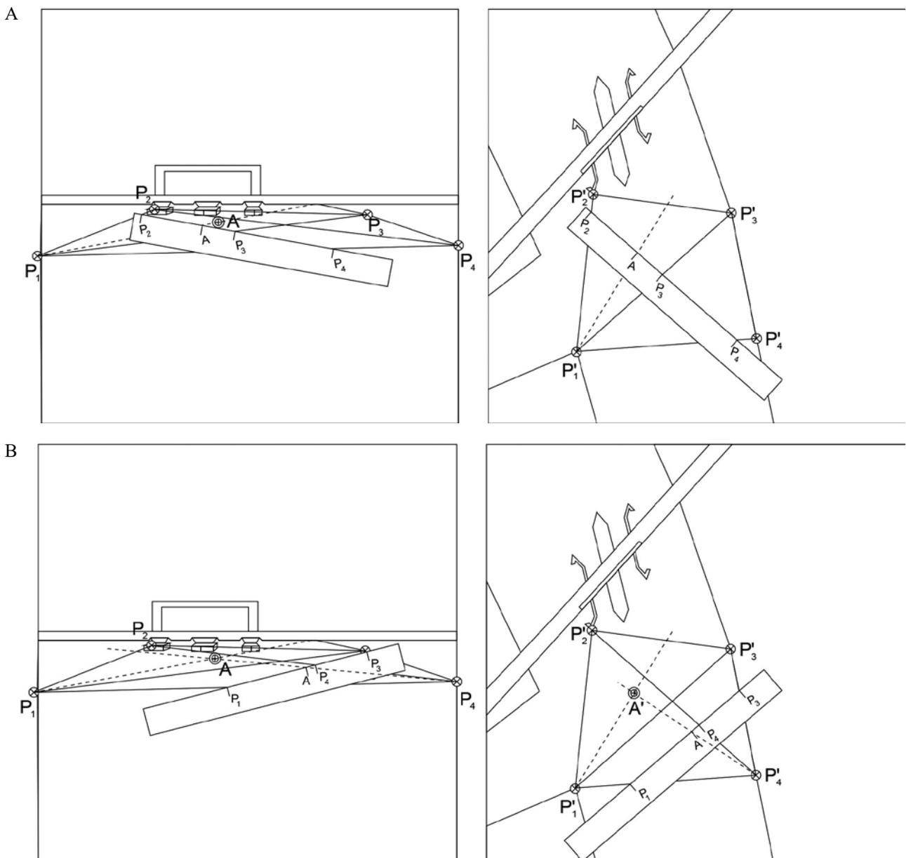
Figure 3. Two steps of the homologous rays method to determine the location of point A'
