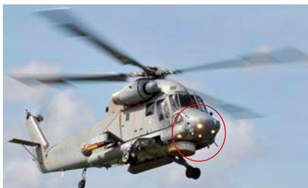
Figure 3. Kaman SH2G “Seasprite” helicopter adapted for the needs of search and rescue missions with an installed floodlight (Wikipedia.pl)
