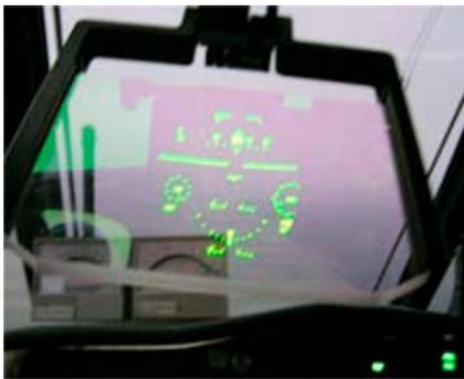
**Figure 6. Piloting-navigational and targeting parameters imaging on a head-up display (HUD) of the W3PL "Głuszec" helicopter (AFIT)**
