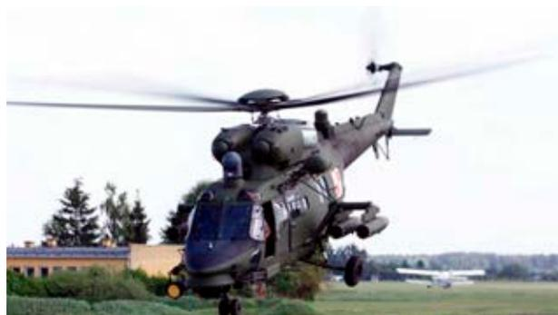
Figure 5. W3PL “Gluszec” helicopter with an integrated avionics system cooperating with a digital observation-targeting head and a moving turret gun position (AFIT)
