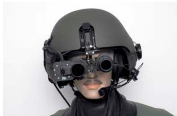
**Figure 12.** NWN1 night-time display of the SWPL1 “Cyklop” and night vision goggles mounted on the THL5 helmet (AFIT)
