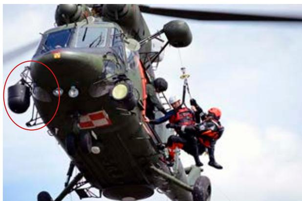
Figure 2. W3WA helicopter adapted for the needs of search and rescue missions with an installed winch (Wikipedia.pl)
