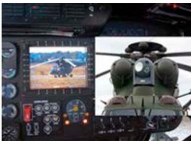
Figure 8. Imaging in daylight from the TOPLITE observation-targeting head displayed on the head monitor for the second pilot-operator of a W3PL "Głuszec" helicopter (AFIT)
