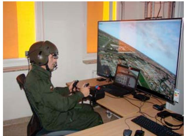
**Figure 15. The flight simulator with a helmet-mounted flight parameter imaging system (AFIT)**
